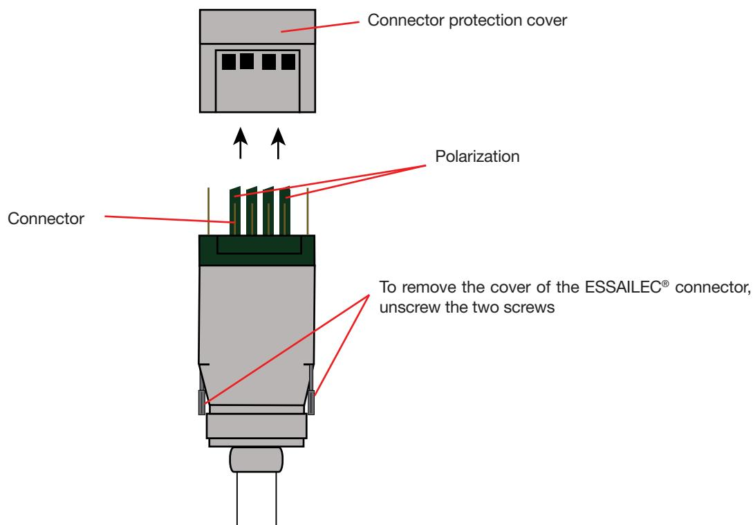
To start the measurements, connect the voltage output connectors to the current terminals of the power and energy analyzer. It automatically recognizes the ESSAILEC® test block.
