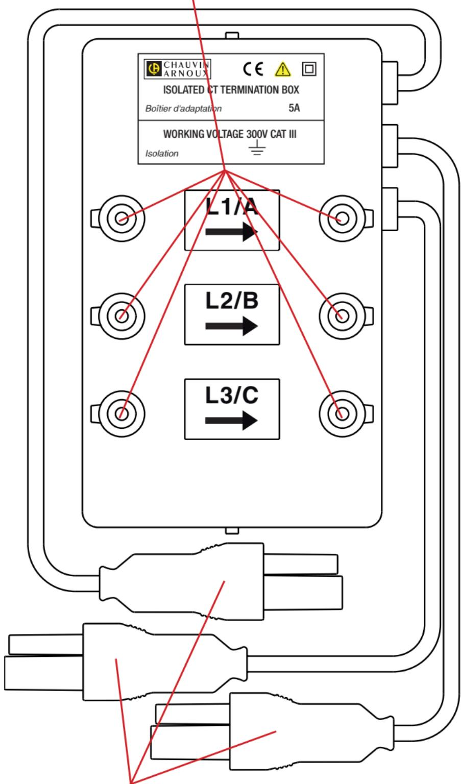
Plugs for connection to the power and energy analyser.
